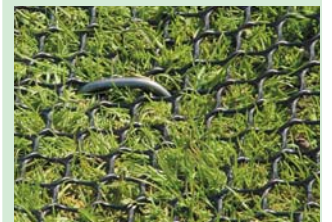
Mesh secured at <1m intervals using steel U-Pins or plastic pegs
